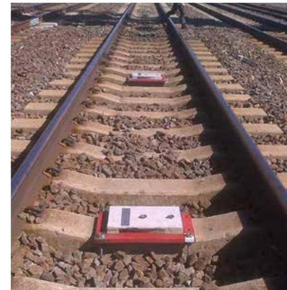
**Transponders mounted between the rails communicate train locations and speeds between on-board computers and signals.**
