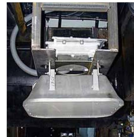
**An antenna mounted under each Amtrak unit picks up information from the transponders.** *Two photos, Amtrak*
