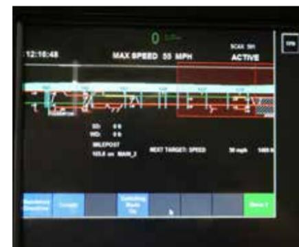
A cab display in service on Metrolink, which started using PTC in February.
